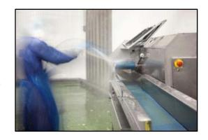
water and caustic chemicals. While TTO coders are usually classified as sensitive equipment (which do not directly touch food and therefore are subject to less stringent cleaning), TTO machines are still susceptible to damage due to their integration in the packaging line.
