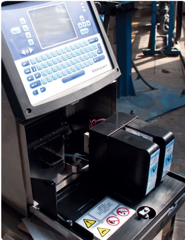
The Smart Cartridge™ fluid delivery system in Baosheng's new Videojet 1710 coder
