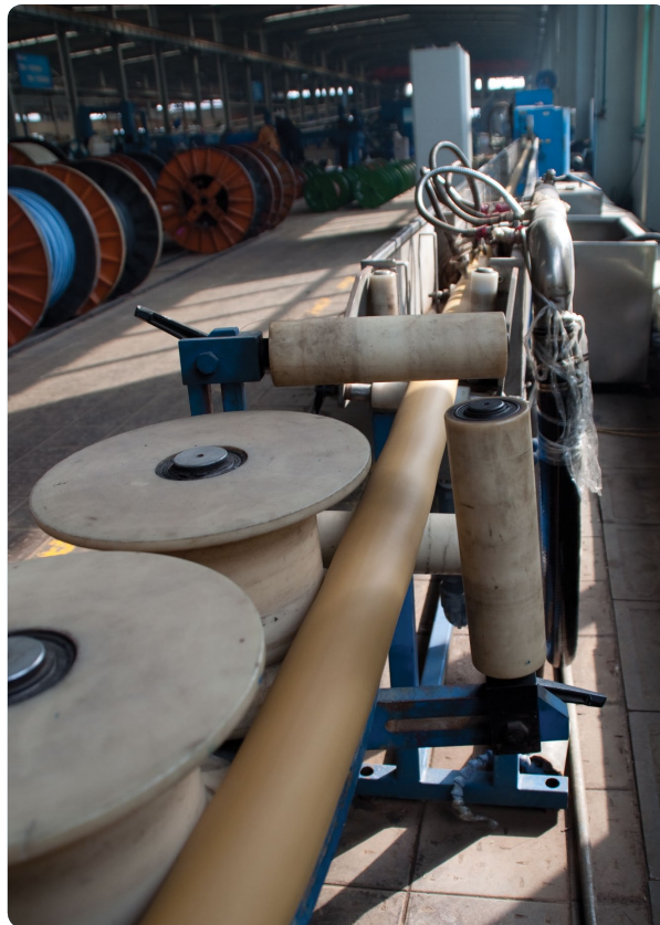
Large-diameter cable production on one of Baosheng's lines
