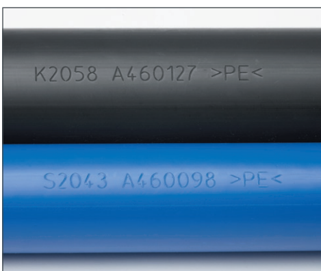
Left: PE tubes. Material effect: engraving. Laser marked with a 50W CO2 laser marker.
