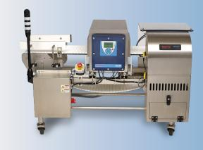
**Thermo Scientific Quickfit**Standard Conveyors for Metal Detectors
