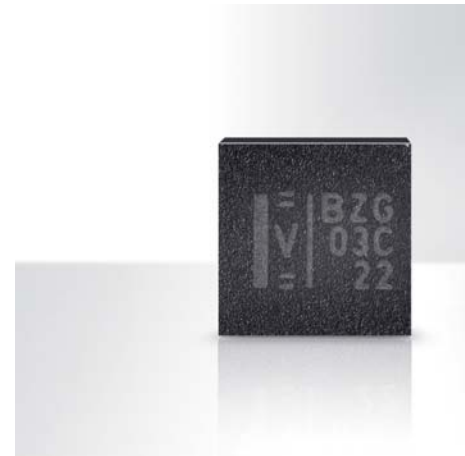
Marked component Marking field: 4 x 4 mm, Marking time: 45 ms
