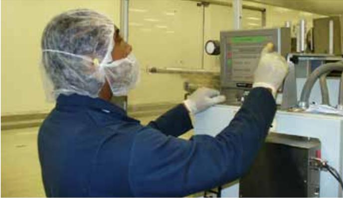
"I used to spend a lot of time calibrating the ink jet printers, but with the Videojet DataFlex printers, I just change the ribbon and use a cotton swab to wipe the printhead, and that's pretty much it," he says.
