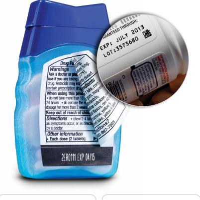
Laser may be utilized to ablate specially preprinted "mark windows" on labels, offering crisp codes and low operating costs from limited required consumables.
