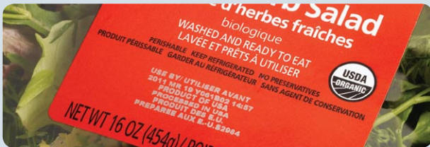
Thermal transfer (TTO) on paper label
