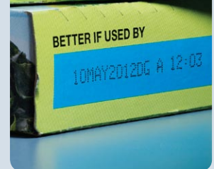
Ink jet and laser on paperboard
