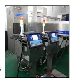
This location is also the most challenging from a speed, space and environmental perspective. At a grader speed of 45 m/min, the printer has about 40 m/sec to print on an egg, whether printing pole-to-pole or across the top of the egg. In this time, the CIJ printer can print two lines of text.
