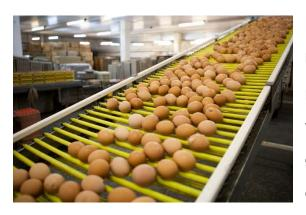
Maintenance requirements are highly correlated to the location of the coding equipment and to the cleanup procedures. In-line egg coding just downstream of the transfer area is potentially the messiest area, since graders often eject eggs in this area, eggs sometimes slip out of the grippers and water and leakers often drip. It is
