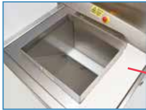
Infeed funnel with adjustable product metering
