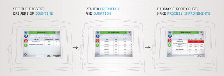
The 1550 and 1650 CLARiTY™ interface presents fault information in a logical way that allows you to identify and focus on the biggest issues and drill down to discover the root causes of unplanned downtime.
