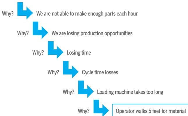
To verify that the analysis is correct, you should be able to propose a countermeasure to the root cause and apply the word "therefore" to verify that the countermeasure addresses each cause in the chain. In this example, moving the material closer to the operator (the countermeasure) reduces walking. Therefore, the machine can be loaded faster. Therefore, cycle time losses are reduced. Therefore, increased time is available. And so on.
