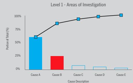
In this chart, the size of each bar shows its contribution to each cause of the problem, and the line plots the operational improvements that can be achieved by addressing each cause. Cause A and cause B clearly have the greatest impacts, and removing them first brings the greatest potential for improvement.
