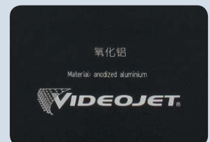
Anodized aluminum: color removal
