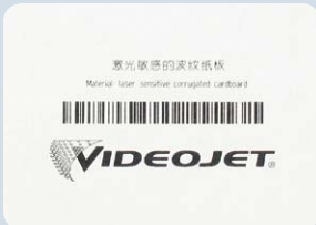
Laser sensitive corrugated cardboard: color change
